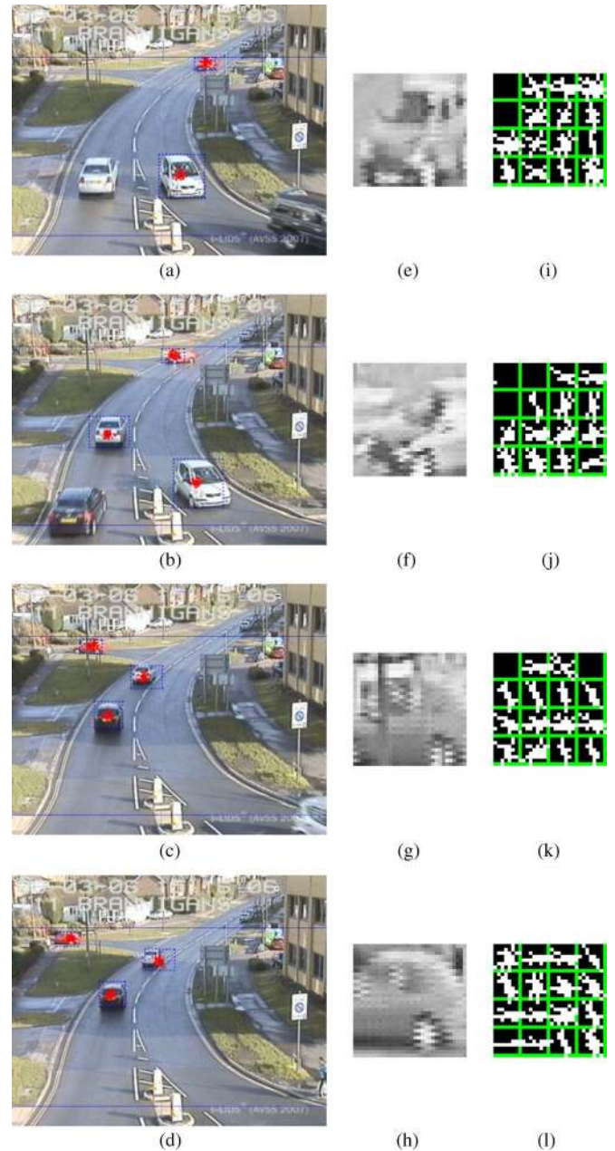
Fig. 14. RDHOGPF tracking results for the red car showing the appearance and RDHOG descriptor updating. (a) Tracking of the red sedan was initiated. (b) Red sedan started to change direction at the crossroads. (c) Red sedan was partially occluded by the utility pole. (d) Presented RDHOGPF method tracked the red sedan until the end of the video. (e)–(h) Appearance of the tracked red sedan. (i)–(l) Corresponding updated RDHOG descriptors.
