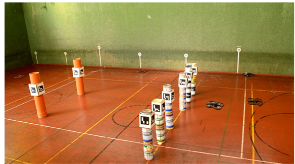
Fig. 1 Experimental flight of a basic instance of the framework “CVG Quadrotor Swarm”. This basic instance is characterized by swarm behavior, using 5 AR Drones. The row of columns represents a virtual wall with a single 1.5 m opening in the middle. In order to simplify the localization problems the columns are marked using ArUco visual markers [5]. In this flight the mission of the swarm is to cross from one side to the other, while each swarm agent also has to avoid collision with the columns and the other drones. This test was designed to showcase the capabilities of this basic instance of the framework
