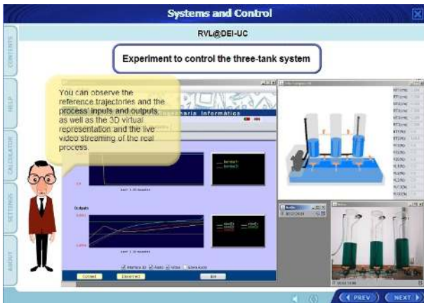
Figure 9. Systems and Control course interacting with the RVL in a three-tank system control experiment.
