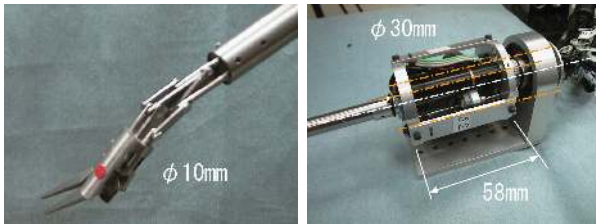
Fig. 3. Link driven multiple DOF forceps
