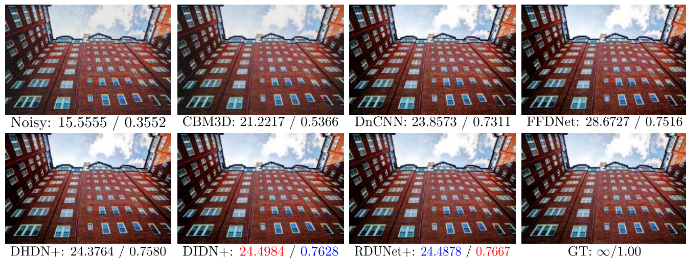
FIGURE 10. Comparison of denoising neural networks. img_034 image from Urban100 dataset corrupted by AWGN with \sigma = 50 . Their corresponding PSNR (dB)/SSIM values of denoised images are shown.
