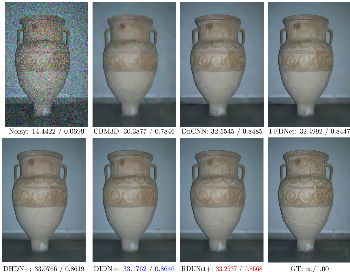
FIGURE 6. Comparison of denoising neural networks. 227092 image from CBSD68 dataset corrupted by AWGN with \sigma = 50 . Their corresponding PSNR (dB)/SSIM values of denoised images are shown.
