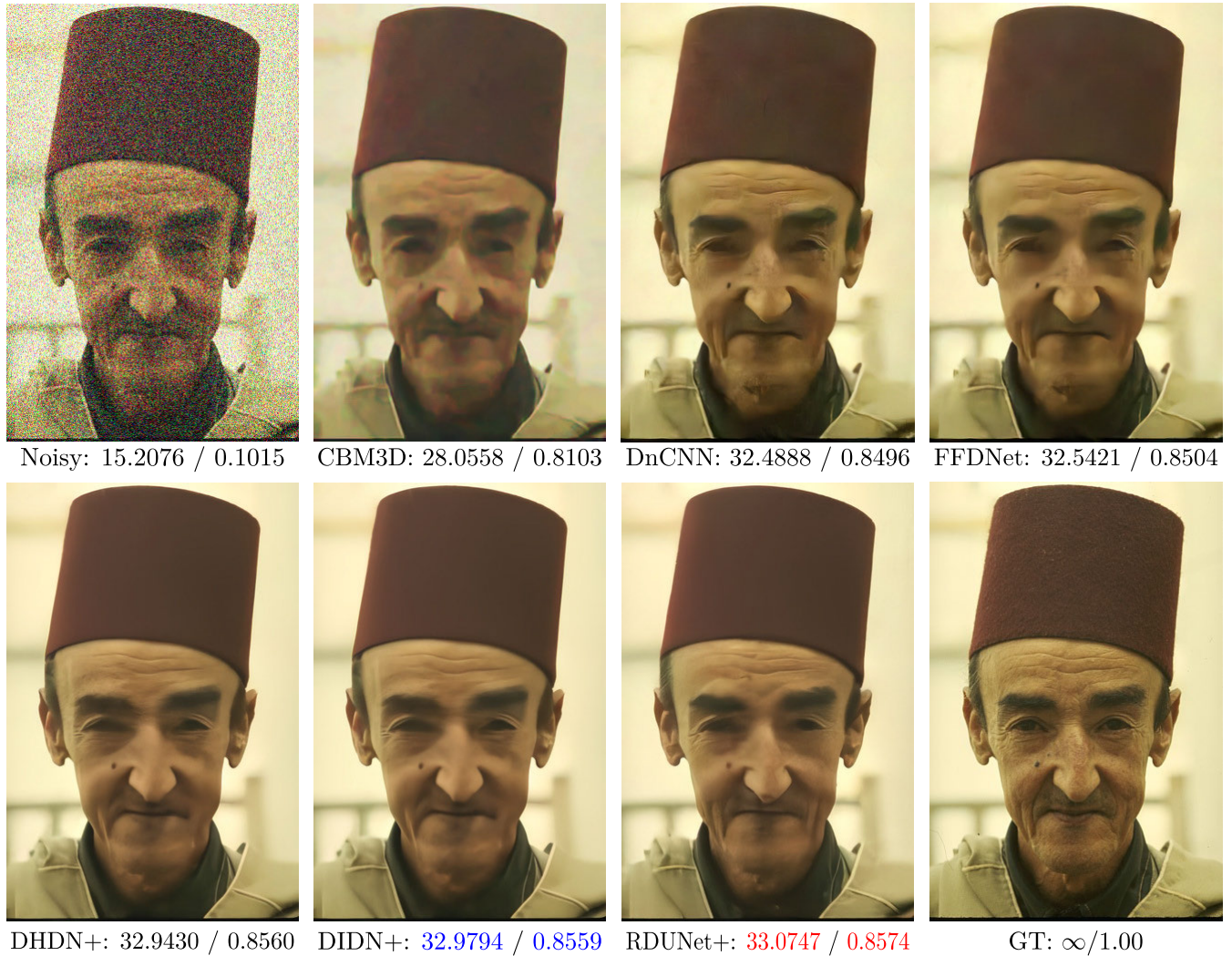
FIGURE 5. Comparison of denoising neural networks. 189080 image from CBSD68 dataset corrupted by AWGN with \sigma = 50 . Their corresponding PSNR (dB)/SSIM values of denoised images are shown.
