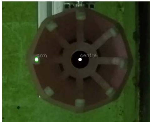
Figure S3: Constrained test image example. These images are used to measure the deflection amplitude and phase of the prototype arms.
