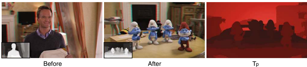
Fig. 1 A scene cut (from The Smurfs 2 © 2013 Sony Pictures Animation Inc., left and middle), with disparity maps of the left view inset, and corresponding per-pixel response time map (right); brighter red indi-
