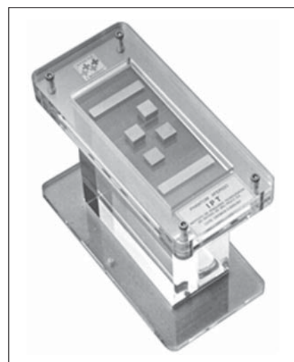
Figure 1. Cromox® reference phantom in bone absorptiometry constructed with bone specimens measured in the IPT metrology laboratory, and utilized for Cromox® devices calibration.
