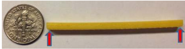
Fig. 9 Simple bar test part with double thickness
