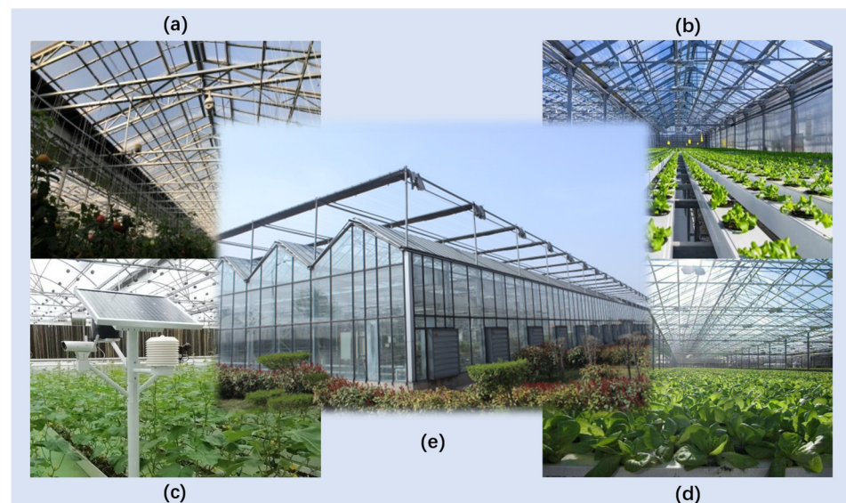
Figure 1. Schematic diagram of data collection environment. (a–d) show the sensors used to collect data on temperature, humidity, light, CO 2 , and light intensity at the top, ground, front, and back of the greenhouse, respectively; (e) shows a panoramic view of the greenhouse.
