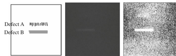
(b) Difference in highlighting two types of defects A and B (left) between conventional setup (middle) and proposed system (right)
