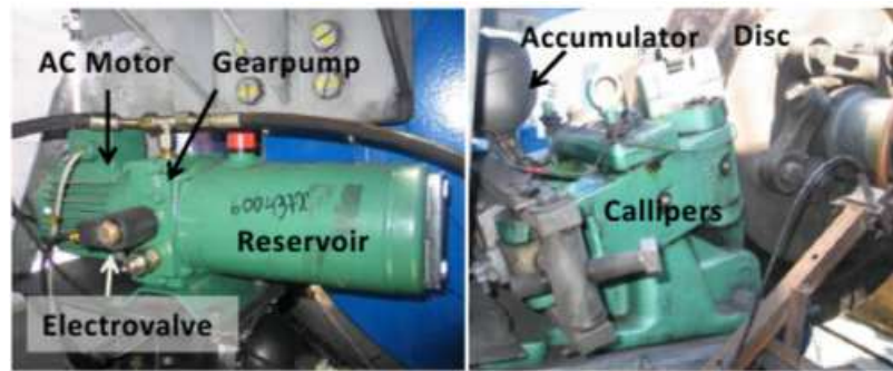
Figure 8. Example of wind turbine brake system [24] [24]
