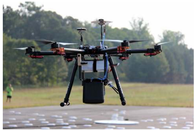
Fig. 4 Close up of Langley Hex Flyer in flight with aerial speaker mounted directly underneath [83]
