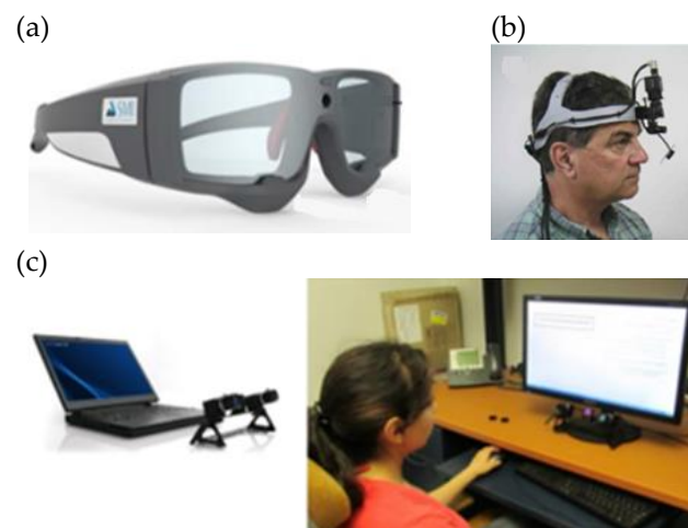
Figure 6. Sample of various kinds of eye-tracking tools: (a) eye-tracking glasses [314]; (b) helmet-mounted [315]; (c) remote or table [316].
