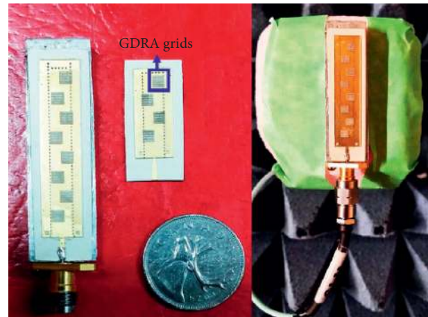
FIGURE 12: Illustration of the 1 \times 8 (on the left) and 1 \times 4 (on the right) GDRA arrays realized in [83] ©2019 IEEE.
