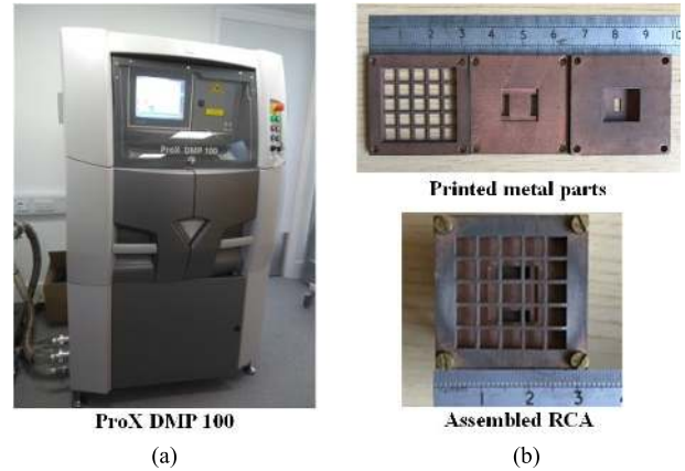
FIGURE 23. The printer and printed antenna.
