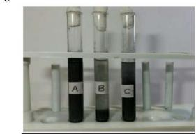
**Fig. 3 a** Three samples immediately after preparation showing no sedimentation. **b** Sample results after 15 h for the same three samples showing least sedimentation in sample A
