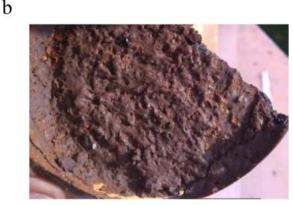
**Fig. 4 a** Interior wall incrustation. **b** Incrustation at the bottom of the container
