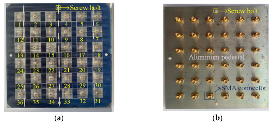
Figure 29. Proposed antenna integrated with solar cell: (a) top view; (b) bottom view [122].
