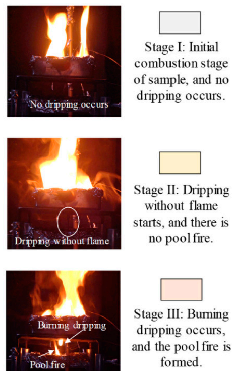
Figure 7. Stage I: combustion with no dripping; Stage II: dripping with no flame; Stage III: burning and dripping; Stage IV: formation of pool flame [15].
