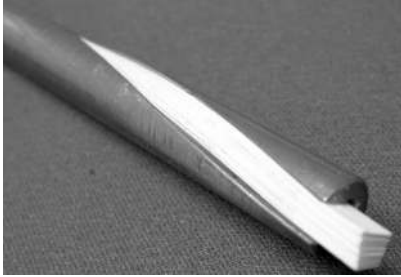
Figure 18. Twisted stack of coated conductor tapes in a grooved copper profile. Reproduced with permission from [138].
