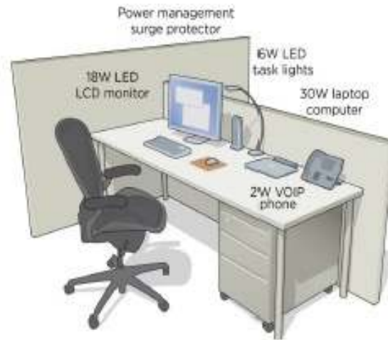
Figure 14. Energy-efficient workspace used for a net zero energy building at the National Renewable Energy Lab Source: (Metzger, Cutler, & Sheppy, 2012)
