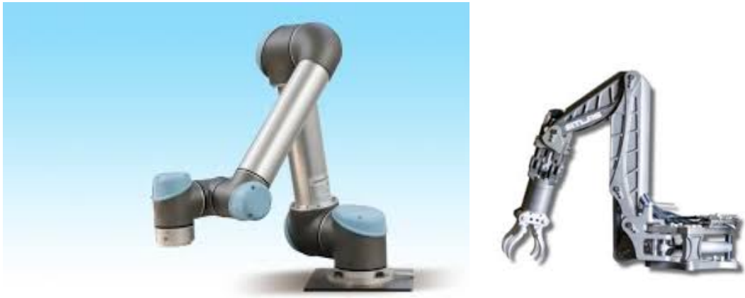
Fig. 22: Two 6R industrial robots with 3 parallel axes: the UR10 robot from Universal Robots (left) and the Schilling Titan II robot (right).
