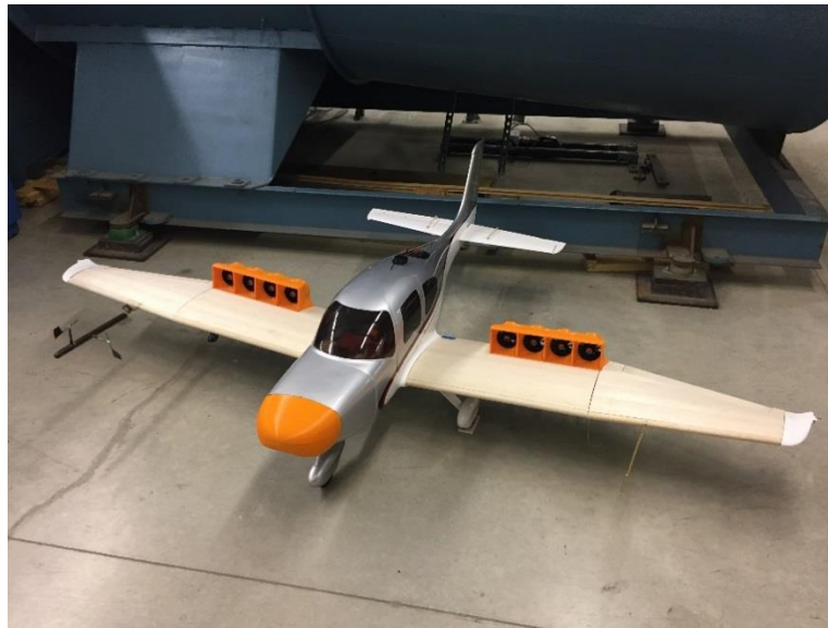
Fig. 9. University of Illinois 21 percent-scale Cirrus SR22T distributed electric propulsion testbed for propulsion-based control (Figure courtesy: University of Illinois at Urbana-Champaign, Urbana, Illinois).
