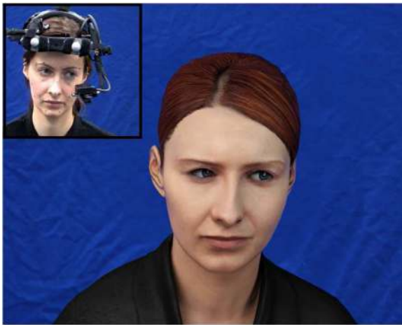
Figure 3: Eye movement capture using a head-mounted eyetracking device, and corresponding virtual avatar displaying the recorded eye movements [MBB12].
