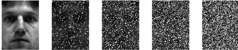
Fig. 6: An aligned face image of Subject 1 in Multi-PIE, Session 1, under the ambient lighting condition (No. 0) is shown on the left. On the right, 20%, 40%, 60%, and 80% of image pixels are randomly selected and corrupted with uniformly distributed values in [0, 255] , respectively.
