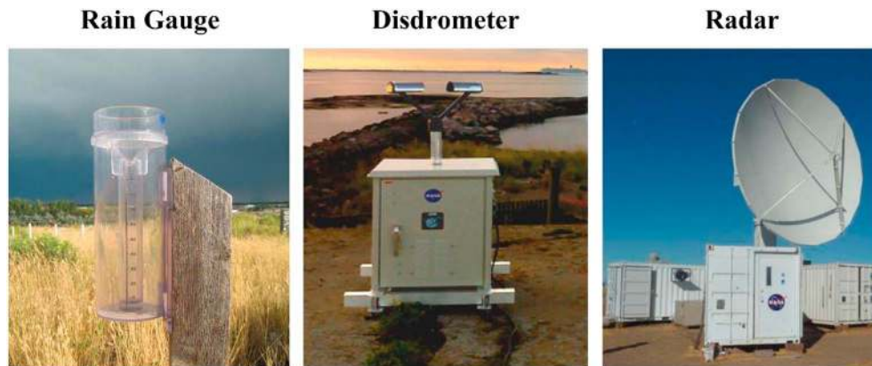
Figure 1. Three instruments for making ground observations of precipitation. Figure adapted from the website of National Aeronautics and Space Administration (NASA) ( https://pmm.nasa.gov/image-gallery/cocorahs-rain-gauge-storm ; https://pmm.nasa.gov/science/ground-validation/ground-instruments ).
