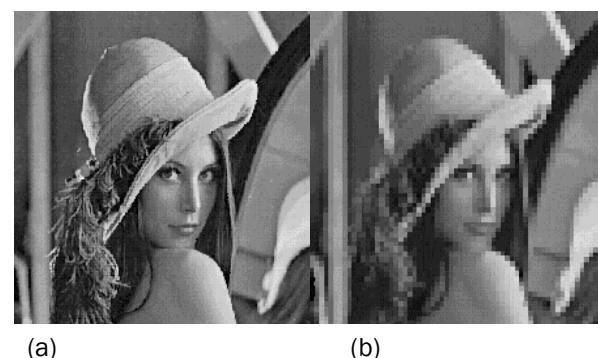
Fig.1:(a) Original Lena Image, and (b) Reconstructed Lena with DC component only, to show blocking artifacts.
