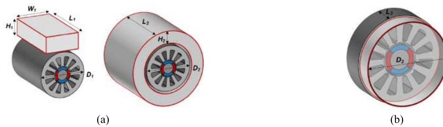
Fig. 4. Different integration methods of power electronics depending on the structure of the electric motors (space for power electronics highlighted in red). (a) Radially mounted for sausage-type motors ( L_1 > D_1 and L_2 > D_2 ). (b) Axially mounted for pancake-type motors ( D_3 > L_3 ).
