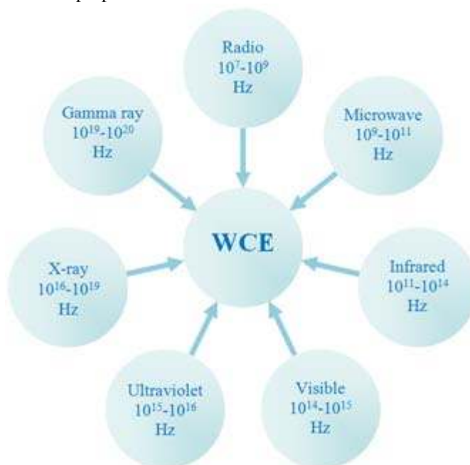
Fig. 7. Utilization of different electromagnetic waves for WCE localization
