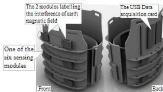
Fig. 3. Wearable sensing modules by Wu et al. [42].
