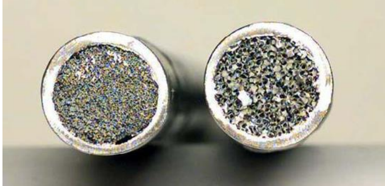
Fig. 10. Metal-foam filled tubes using co-sintering technique [68].
