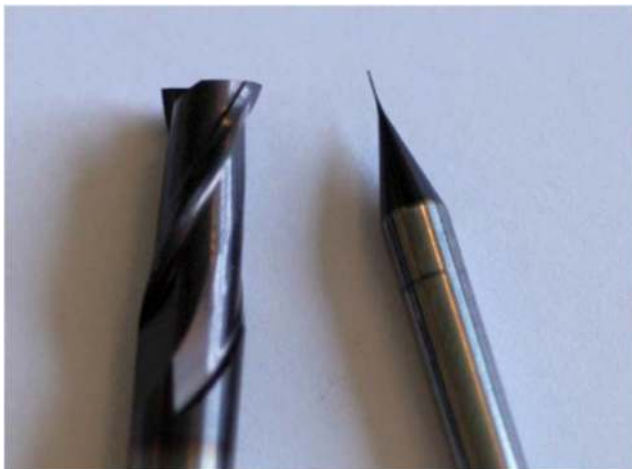
Fig. 15 Optical photograph illustrating the difference in scale between milling (left) and micro-milling (right) tools [105]
