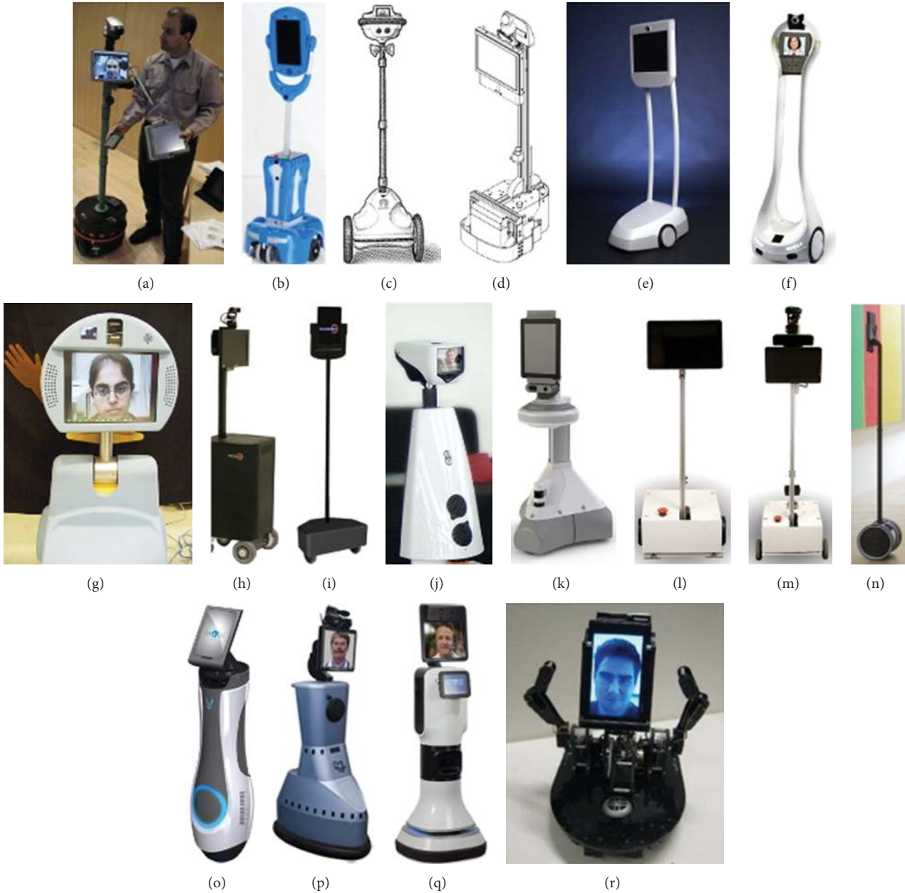
FIGURE 1: (a) PRoP, (b) Giraff, (c) QB, (d) Texai, (e) Beam, (f) VGo, (g) PEBBLES, (h) MantaroBot Classic, (i) MantaroBot TeleMe, (j) Jazz Connect, (k) iRobot Ava, (l) 9th Sense Helo, (m) 9th Sense Telo, (n) Double, (o) mObi, (p) RP-7, (q) RP-VITA, and (r) MeBot.
