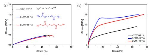
**Figure 48.** Mechanical properties of DLP 3D printed materials (**a**) prior to and (**b**) after thermal treatment at 180 °C for 4 h. Reproduced with permission from [101]. Copyright © 2022 Elsevier.
