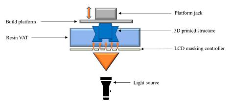
Figure 7. Schematic diagram of the liquid crystal display (LCD) printing process.
