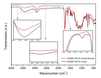
**Figure 47.** ATR-FTIR spectra of thiol-acrylate 3D printed samples prior to and after thermal annealing at 180 °C for 4 h. Inset plots present zoomed images of the -OH (3600–3200 cm $^{-1}$ ), -SH (2600–2500 cm $^{-1}$ ), and C=C-H (1700–1600 cm $^{-1}$ ) absorption bands before and after thermal annealing. Reproduced with permission from [101]. Copyright © 2022 Elsevier.
