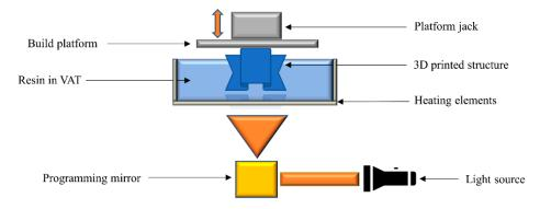
**Figure 9.** Schematic diagram of the hot lithography process.
