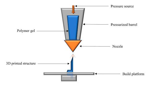
Figure 3. Schematic diagram of the direct ink writing (DIW) process. Redrawn from [10].
