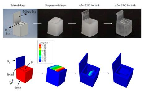
**Figure 40.** (**Top**) 3D printed box with two lids. The box opens at 52 °C and closes at 58 °C. (**Bottom**) Results of the finite element simulation. Red and blue colors in the first figure on the left denote pure and mixed ink, respectively. Reproduced from [70].
