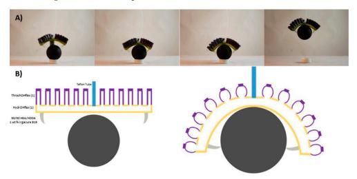
**Figure 43.** (**A**) Multi-material 3D printed pneumatic gripper, descending, pneumatically actuating, and grabbing a plastic ball. (**B**) Schematic illustration of the multi-material gripper before (**left**) and after (**right**) pneumatic actuation. Ball diameter = 38 mm. Reproduced from [347].
