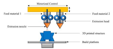
**Figure 11.** Schematic diagram of the multi-material FFF process. A central motorized controller adjusts the position of the extrusion heads intermittently for layer-by-layer extrusion of each material.
