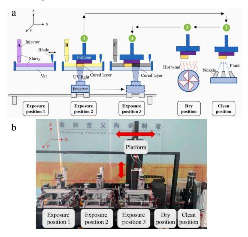
**Figure 30.** (a) Conceptual diagram of multi-material DLP 3D printing setup and (b) overview of the actual multi-material DLP 3D printer developed by Hu and co-workers. Reproduced with permission from [63]. Copyright © 2022 Elsevier.
