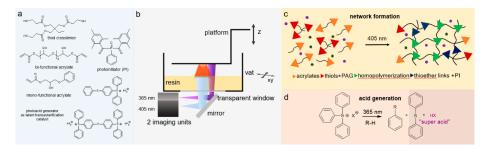
**Figure 34.** (a) Constituents of the resin formulation for selectively activating a transesterification catalyst in thiol-acrylate photopolymers; (b) dual-light wavelength DLP 3D printer setup; (c) visible light-mediated network formation during DLP 3D printing; (d) UV light-triggered activation of Brønsted acids acting as a transesterification catalyst. Reproduced from Ref. [237] with permission from the Royal Society of Chemistry.
