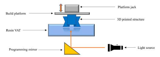
Figure 5. Schematic diagram of the stereolithography (SLA) process.
