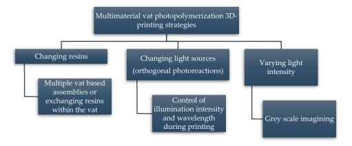
Figure 25. Strategies for multi-material vat photopolymerization 3D printing.
