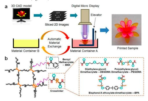
**Figure 28.** (a) Process working schematics for multi-material SLA printing using two different monomers and (b) the chemical structure developed by monomers via multi-material SLA printing. Reproduced from [61].
