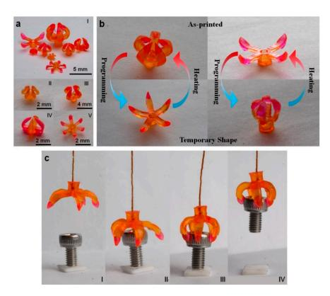
**Figure 41.** 3D printed multi-material grippers: (a) different sizes and designs of 3D printed grippers; (b) illustration of transitions between printed and temporary shapes as a function of temperature; (c) gripper used to lift a bolt assembly. Reproduced with permission from [61].
