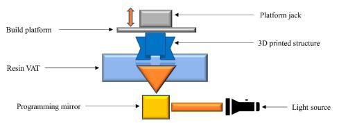
Figure 6. Schematic diagram of the digital light processing (DLP) process.
