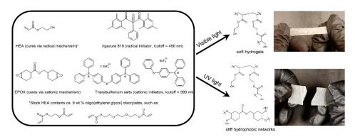
**Figure 32.** Representation of MASC strategy to achieve different networks with discrete wavelengths of light irradiation. A stiffer network was formed by cationic epoxy polymerization, while a softer network was generated by radical acrylate polymerization. Reproduced from [320].
