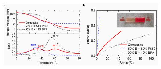
**Figure 50.** Thermomechanical tests to investigate the interface bonding within multi-material structures (Material A = 50%B + 50%P550; Material B = 90%B + 10%BPA): (a) DMA and (b) uniaxial tensile tests of the composite and the single materials [61].
