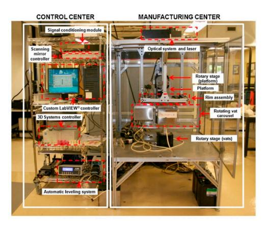
**Figure 26.** Multi-material SLA setup developed by Choi and coworkers, reproduced with permission from [57]. Copyright © 2022 Elsevier.
