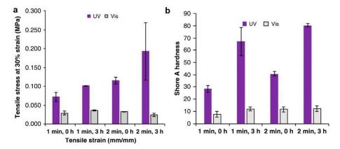
**Figure 46.** (a) Tensile stress values at 30% strain for UV and vis-light cured samples; (b) Shore A hardness of UV and vis-light cured samples. Time in minutes represents illumination times and time in hours represents times of thermal post-curing [320].
