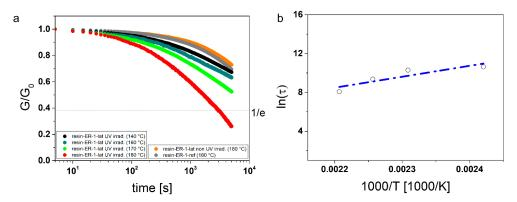
**Figure 45.** (a) Normalized stress relaxation behavior of multi-materials over time at various temperatures; (b) Arrhenius plot of UV-activated multi-materials derived from measured relaxation times. Reproduced from Ref. [237] with permission from the Royal Society of Chemistry.
