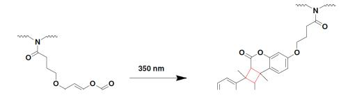
**Figure 53.** Coumarin side-groups undergoing  $[2\pi + 2\pi]$  cycloaddition reaction upon UV irradiation. Reproduced with permission from [375]. Copyright © 2022 Elsevier.
