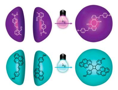
**Figure 55.** Purple area: o-MBA ( $\lambda_1$  maximum = 330 nm purple); turquoise area: StyP ( $\lambda_2$  maximum = 435 nm): activations for implementing a  $\lambda$ -orthogonal photoresist. Reproduced with permission from [364]. Copyright © 2022 John Wiley and Sons.
