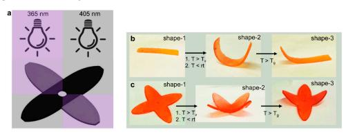
**Figure 44.** (a) Illustrations of the printing setup of the rectangular bar and grippers; (b) the permanent, programming, and spatially-controlled shaping experiment; and (c) the permanent, programming, and spatially-controlled state of the multi-material gripper under thermal stimuli. Reproduced from Ref. [237] with permission from the Royal Society of Chemistry.
