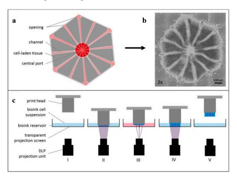
**Figure 37.** Cell brick 3D printing process of liver: (a) virtual 3D design; (b) microscopic image of the printed multi-material cell-laden hydrogel; (c) multi-material DLP 3D printing setup used for liver design printing. Reproduced from [329].
