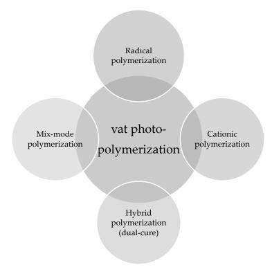
Figure 13. Reaction strategies for vat photopolymerization 3D printing.
