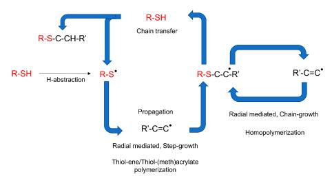
**Figure 24.** Reaction cycle representing mixed-mode thiol-ene and acrylate homopolymerization. Active carbon centers can participate in chain transfer as well as chain propagation. Reproduced with permission from [225]. Copyright © 2022 John Wiley and Sons.
