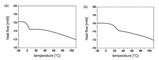
**Figure 49.** DSC plots of vat photopolymerized thiol-acrylate resins (**a**) prior to and (**b**) after thermal post-treatment at 180 °C for 4 h. Reproduced from Ref. [102] with permission from the Royal Society of Chemistry.
