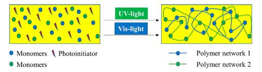
**Figure 31.** Conceptual illustration of orthogonally-evolved photopolymer networks via two different types of light illumination. Polymer Network 1 forms the first layer and polymer Network 2 forms the second layer for subsequent building of multi-material structures.
