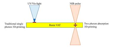
**Figure 10.** UV light is absorbed at the surface of a photosensitive resin, and can only be used for fabrication of planar structures (one-photon absorption). NIR light is focused into the volume of the photocurable resin and is used for 3D structuring (TPP). Reproduced with permission from [123]. Copyright © 2022 Elsevier.
