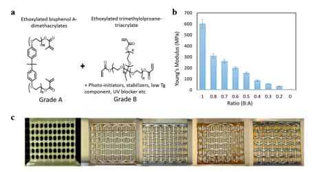
**Figure 36.** (a) Components of resin formulation; (b) tunable stiffness bandwidth in photocured polymers by varying concentration of A and B components; and (c) physical representation of printed architectures with varying compositions. Reproduced from [327].
