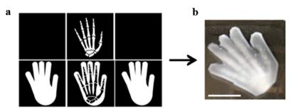
**Figure 35.** (a) Arbitrary scale DLP projection images; upper design (bones) printed with UV light, lower design printed with visible-light. (b) Multi-material DLP 3D printed hand using UV and visible light projections. Scale bar represents 25 mm. Reproduced from [320].
