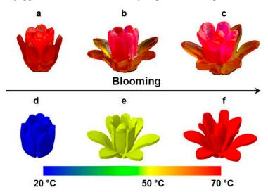
**Figure 42.** Stimuli-responsive behavior of a multi-material 3D printed flower: (a) Programmed (temporary) shape of the multi-material flower held at 20 °C; (b) heating to 50 °C, resulting in the flower's outer buds opening; (c) the flower fully bloomed at 70 °C; (d–f) simulation images of the complete multi-material flower blooming process. Reproduced with permission from [61].
