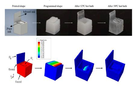
**Figure 29.** Thermally-induced transitions in a double-lid multi-material DLP printed box. Both lids remain closed below 52  $^{\circ}$ C; at 52  $^{\circ}$ C, both lids open. The inner lid closes at 58  $^{\circ}$ C. Reproduced from [70].
