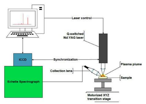
Figure 11. Picture of the LIBS setup [56].
