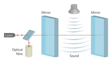
Figure 8. Schematic of the membrane-free optical microphone by Xarion [77].
