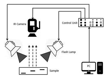
Figure 17. Pulse thermography setup [105].
