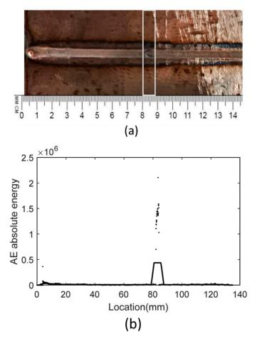
**Figure 9.** A correlation between acoustic emission absolute energy and welding defect [87]. (**a**) depicts the inspected sample. (**b**) shows the acquired AE absolute energy of the inspected weld seam.
