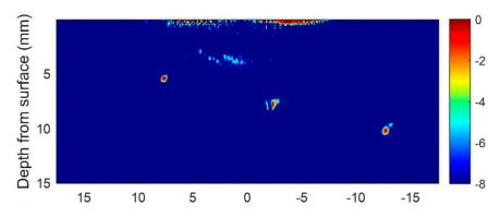
**Figure 4.** Intentionally introduced defects (D1, D2 and D3 in Figure 3) are detected by means of TFM image of the component using ultrasonic longitudinal waves [25].
