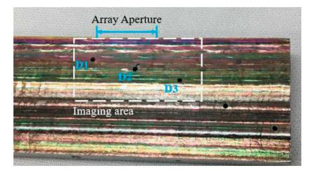
Figure 3. Inspected WAAM component. D1, D2 and D3 represent the welding defects [25].
