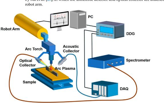
Figure 13 illustrates a possible concept of an online LOUD monitoring system proposed by Ma et al. [28], in which the ultrasonic detector and optical collector are attached to the robot arm.
