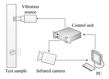
Figure 18. A picture of a vibrothermography setup [116].
