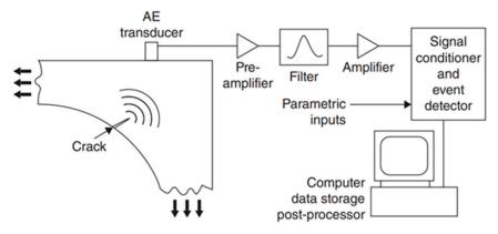
Figure 7. Graphical illustration of a conventional AE measurement system [76].
