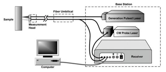
Figure 5. Laser ultrasonic inspection system [48].
