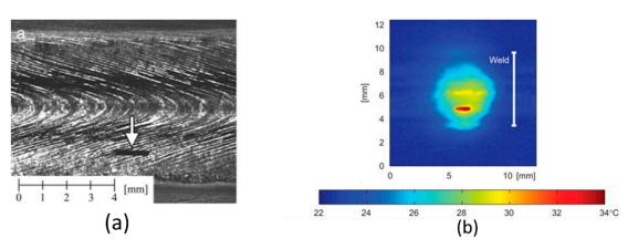
**Figure 15.** Defect detection by means of the thermography technology performed by Broberg [108]. (a) displays the defect (the arrow shows its position). (b) shows the captured thermal image, in which the defect can be recognised.
