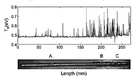
**Figure 10.** A schematic of the OES technique [95]. In this illustration, the recorded electronic temperature is correlated with the existing welding defects (A, B and C).
