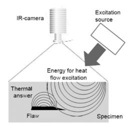
Figure 16. A schematic of active thermography [106].
