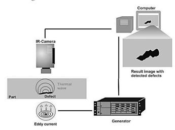
Figure 19. An illustration of eddy current thermography [118].
