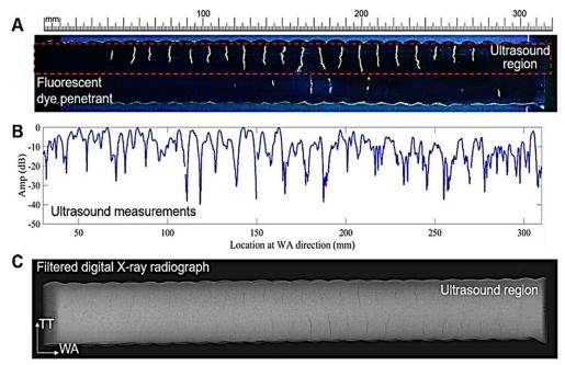
Figure 2. A comparison between dye penetrant testing (the dashed section in (A) depicts the area examined with ultrasound techniques shown in (B)) (A), conventional ultrasonic (B) and X-ray radiographic technologies (C) carried out by Seow et al. [20].
