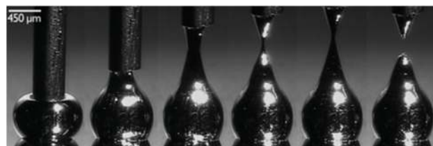
Fig. 5 Above: Sequential images showing formation of an EGaIn tip by withdrawal of a syringe needle filled with EGaIn from a drop of EGaIn on a silver surface. This figure has been reproduced from ref. 17 with permission from Wiley-VCH, copyright 2008. Below: Cartoon of an EGaIn tip contacting a SAM of molecules of interest on a Au surface. Lighter grey spheres represent the Ga_2O_3 oxide layer that coats the EGaIn (darker grey spheres). The large area of the tip relative to a molecule means multiple molecules bridge the surface-tip gap and contribute to junction conductance.
