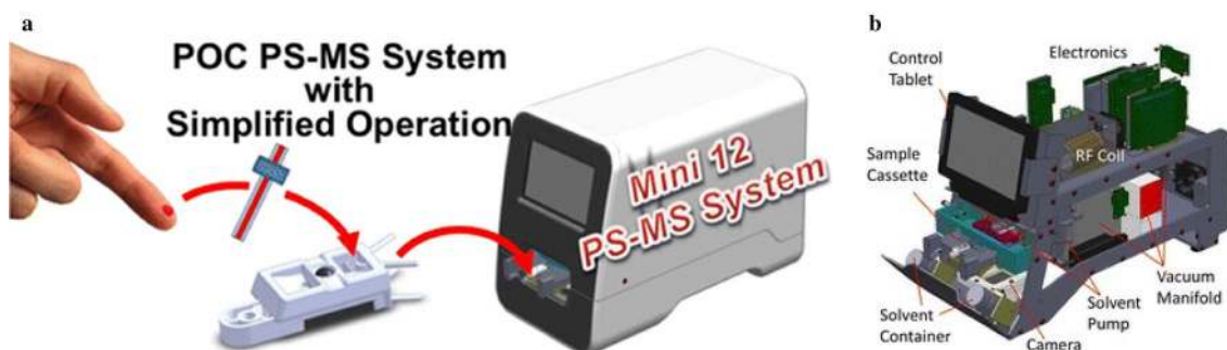
Fig. 12 Mini 12 paper-spray (PS) MS developed by Li et al. [118] a Simplified user operation for point-of-care (POC) applications. b Overview of system components
