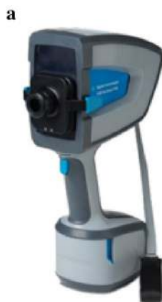
Fig. 2 Agilent 4300 Handheld FTIR spectrometer (Agilent, Santa Clara, CA, USA) a image, b practical use in geological studies. Reproduced from Agilent [11]
