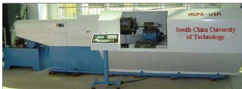
Fig. 33. HGPX-WSM multi-function CNC spinning machine [24].
