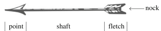
Fig. 6 A quick way to get Re for an arrow is to set D in Eq. 9 equal to the mean shaft diameter. One research group [33] gets drag contributions from the four labeled parts of the arrow
