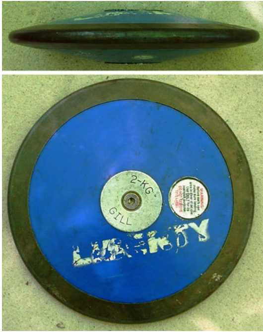
Fig. 9 End view ( top ) of a men's 2-kg discus presents minimum cross-sectional area, which is about one-sixth of the maximum cross-sectional area ( bottom ) of 0.038 \text{ m}^2 ( 0.41 \text{ ft}^2 )
