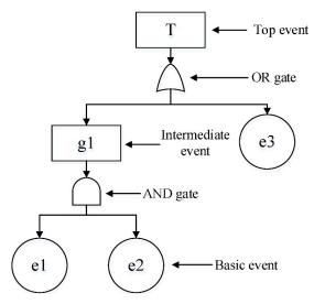
Figure 3. Basic fault tree representation [48].
