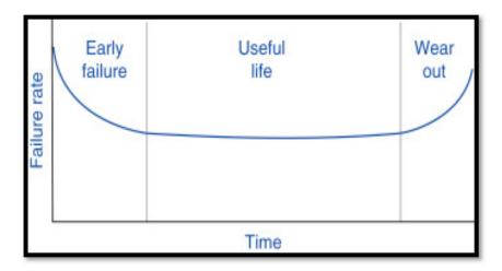
Figure 4. Bathtub curve representing equipment failure rate [60].
