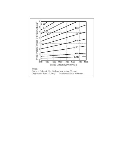
Figure 4: LCOE for energy output versus initial cost of the system for a zero interest loan, discount rate of 4.5%, degradation rate of 0.5%/yr and 30 year lifetime.
