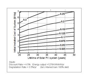
Figure 3: LCOE for lifetime of solar PV system versus initial cost of the system for a zero interest loan, discount rate of 4.5%, degradation rate of 0.5%/yr and energy output of 1270 kWh/kW.
