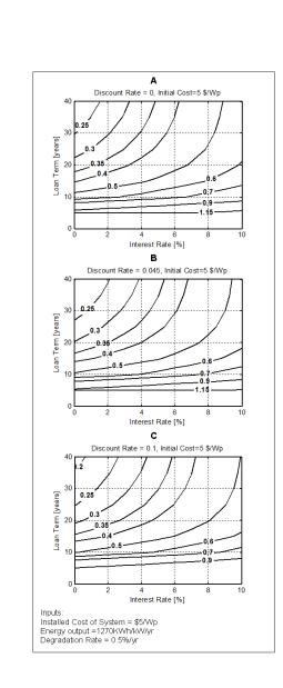
Figure 1: LCOE in \$/kWh for solar PV system varying interest rates, loan terms and discount rates (A: 0%, B: 4.5%, C: 10%) assuming initial installed system cost of \$5/Wp, degradation rate of 0.5%/yr and energy output of 1270 kWh/kW/yr.
