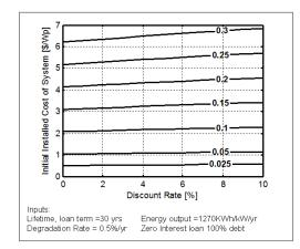
Figure 2: LCOE in \$/kWh for solar PV system varying system costs and discount rates assuming zero interest loan, 30 year lifetime, degradation rate of 0.5%/yr and Energy output of 1270 kWh/kW/yr.
