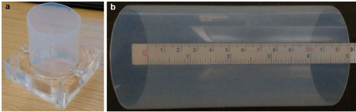
Fig. 8 Photographs of an ETFE pipe with a 50-mm ID and 1-mm wall thickness: a located within a PMMA flange; and b with an internal measurement tape
