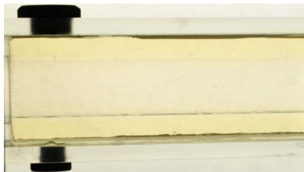
Fig. 6 Fused quartz pipe located inside a correction box with RIM liquid Exxsol D140 (RI = 1.459) both surrounding the box and within the pipe
