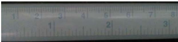
Fig. 9 Photograph of a PVDF pipe with a 14-mm ID and 0.7-mm wall thickness with an internal measurement tape
