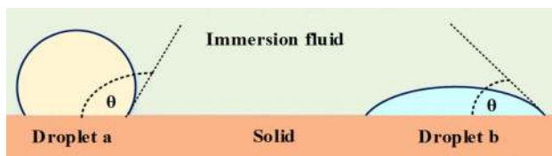
Fig. 4 Two droplets on a solid surface in a lighter emersion fluid ( gas or liquid ) making contact angles \theta with a solid. The liquid of droplet (a) has a lower affinity for the surface than the immersion fluid and, therefore, has a large contact angle, while the liquid of droplet (b) has a greater affinity for the solid than the immersion fluid and so has a smaller contact angle
