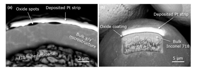
**Figure 18.** Back-scattered electron micrograph of particle with FIB sectioning to reveal microstructure and surface oxides (darker material) for particle (**a**) with oxide spots and (**b**) with oxide coating. The bright section is the sacrificial platinum strip deposited prior to ion milling. (Reprinted with permission from Ref. [66]. Copyright 2018 Elsevier B.V.).
