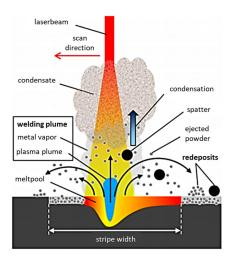
**Figure 16.** Spatter and other by-products pass through the laser stream and squander laser energy, condensate is the product of vaporized metal that quickly cools and condenses. (Reprinted with permission from Ref. [87]. Copyright 2016 Elsevier B.V.).
