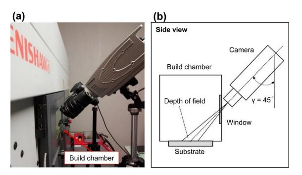
**Figure 5.** Off-axial detection system: (**a**) off-axial mounting of the high-speed camera outside the build chamber; (**b**) off-axial high-speed camera is at an angle of  $45^{\circ}$  to the plane of the observed powder bed. (Reprinted with permission from Ref. [39]. Copyright 2017 Elsevier B.V.).
