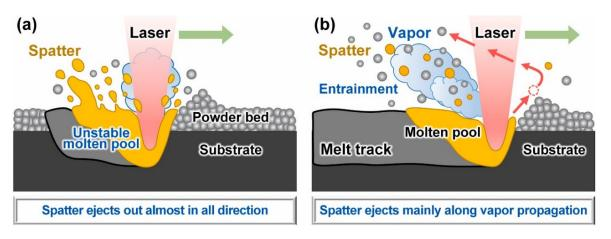
**Figure 13.** Schematic diagram of the transformation of the main mechanisms of spatter generation, which changes from (**a**) the vapor-induced recoil pressure with an almost homogeneous distribution of spatter ejection angle, into (**b**) the vapor-induced entrainment that majority of spatters eject along the direction of the metal vapor propagation. (Reprinted with permission from Ref. [80]. Copyright 2021 Elsevier B.V.).
