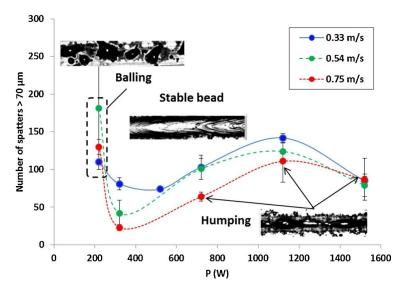
**Figure 22.** On a 316L stainless steel powder bed, the effect of laser power and scanning velocity on large-sized spatter, For low laser powers (P = 220 W) and resulting VED values severe balling occurs, that generates important spattering. The lower amount of spatters is obtained for P values just above the balling threshold (P = 320 W, V = 0.54 m/s and 0.75 m/s). (Reprinted with permission from Ref. [78]. Copyright 2018 Elsevier B.V.).
