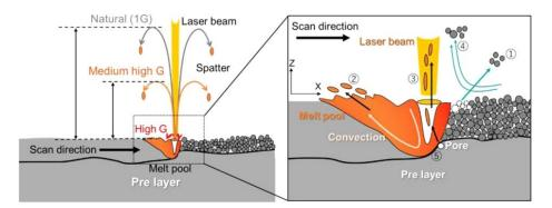
**Figure 26.** Classification and suppression of spatter under high gravitational acceleration: ① solid spatter; ② metallic ejected spatter; ③ powder agglomeration spatter; ④ entrainment melting spatter; and ⑤ defect induced spatter. (Reprinted with permission from Ref. [139]. Copyright 2021 Elsevier B.V.).
