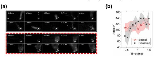
**Figure 23.** (a) Side views of melt pool captured using Gaussian (top, gray border) and Bessel (bottom, dashed red border) lasers; (b) angle of melt pool steam relative to horizontal level as a function of time. (Reprinted with permission from Ref. [129]. Copyright 2021 AAAS).
