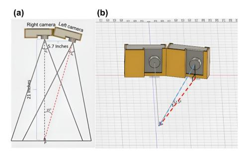
**Figure 6.** Spatter detection system for stereo vision: (a) the horizontal angle between the two sensors is  $15^{\circ}$ ; (b) the vertical direction of the sensor is  $12.5^{\circ}$  from the observation object. (Reprinted with permission from Ref. [43]. Copyright 2018 University of Texas at Austin).
