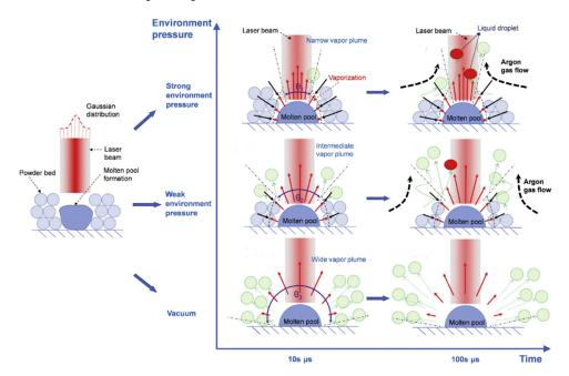
**Figure 24.** Schematic of powder spattering behavior as a function of time and environment pressure during L-PBF.(Reprinted with permission from Ref. [36]. Copyright 2018 Elsevier B.V.).
