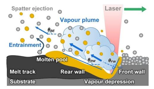
**Figure 11.** Schematic of the correlation between the depression zone in melt pool and the backwardejected spatter during L-PBF. The inclined angles for the normal direction of the front depression wall  $\theta_{FW}$  and the inclination angle of the rear depression wall  $\theta_{RW}$  had the same trends with the average angle of the backward-ejected spatter ( $\theta_{BE}$ ). (Reprinted with permission from Ref. [34]. Copyright 2019 Elsevier B.V.).
