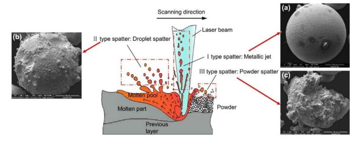
**Figure 8.** Formation mechanisms of different types of spatter during L-PBF: (**a**) morphology of spherical spatter (Type-I spatter); (**b**) morphology of coarse spherical morphology (Type-II spatter); (**c**) morphology of irregular spatter (Type-III spatter). (Reprinted with permission from Ref. [63]. Copyright 2016 Elsevier B.V.).
