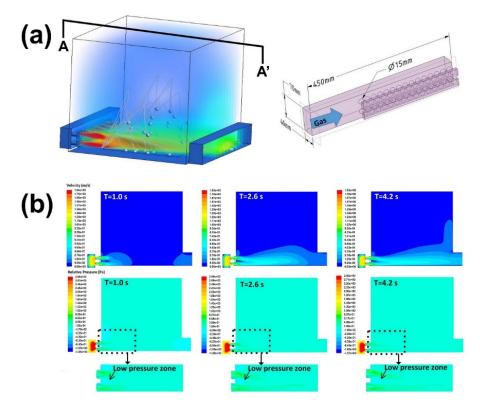
**Figure 27.** CAD model of counter-Coanda effect in L-PBF build chamber: (**a**) the counter-Coanda effect design that employs another row of nozzles directly under the primary nozzles; (**b**) A-A' plane: transient velocity and pressure field. (Reprinted with permission from Ref. [137]. Copyright 2020 Elsevier B.V.).
