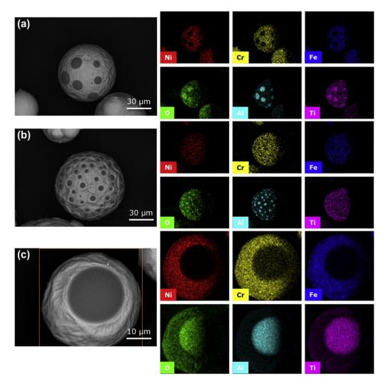
**Figure 17.** Back-scattered electron micrograph, and electron X-ray dispersive spectroscopy mapping of elements of Inconel 718 spatter collected from the ReaLizer SLM50. ( $\mathbf{a}$ - $\mathbf{c}$ ) shows that the dark spots mostly contain Al and O, and that the larger dark spots also contain Ti. EDS quantification results indicated that the oxides were a combination of Al<sub>2</sub>O<sub>3</sub> and TiO<sub>2</sub>. (Reprinted with permission from Ref. [66]. Copyright 2018 Elsevier B.V.).
