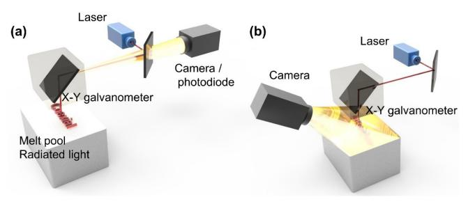
**Figure 4.** L-PBF in situ detection system: (a) coaxial (sharing the optical path with the laser); (b) off-axial (at a slight angle to the laser optical path).
