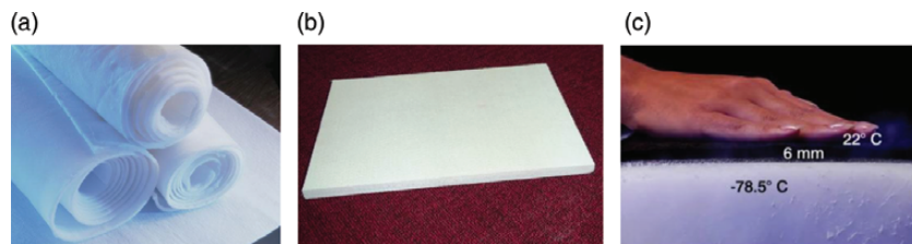
Figure 5. Flexible aerogel blankets and solid aerogel boards. (a) Aerogel blankets [2], (b) aerogel panel [23] and (c) superinsulating aerogel blanket [2].
