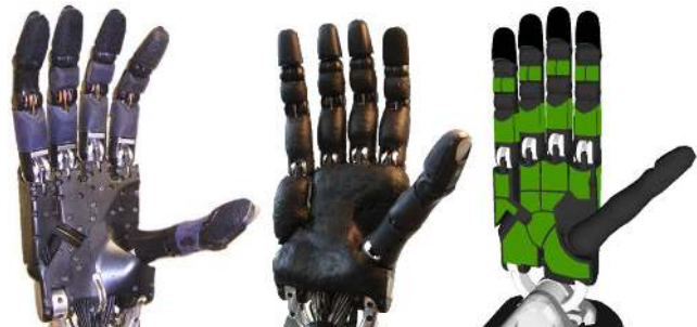
Fig. 2. A Shadow Dexterous Hand (left) that has been covered with a tactile skin (middle) in order to provide tactile information at several locations (highlighted green regions on the right rendering).
