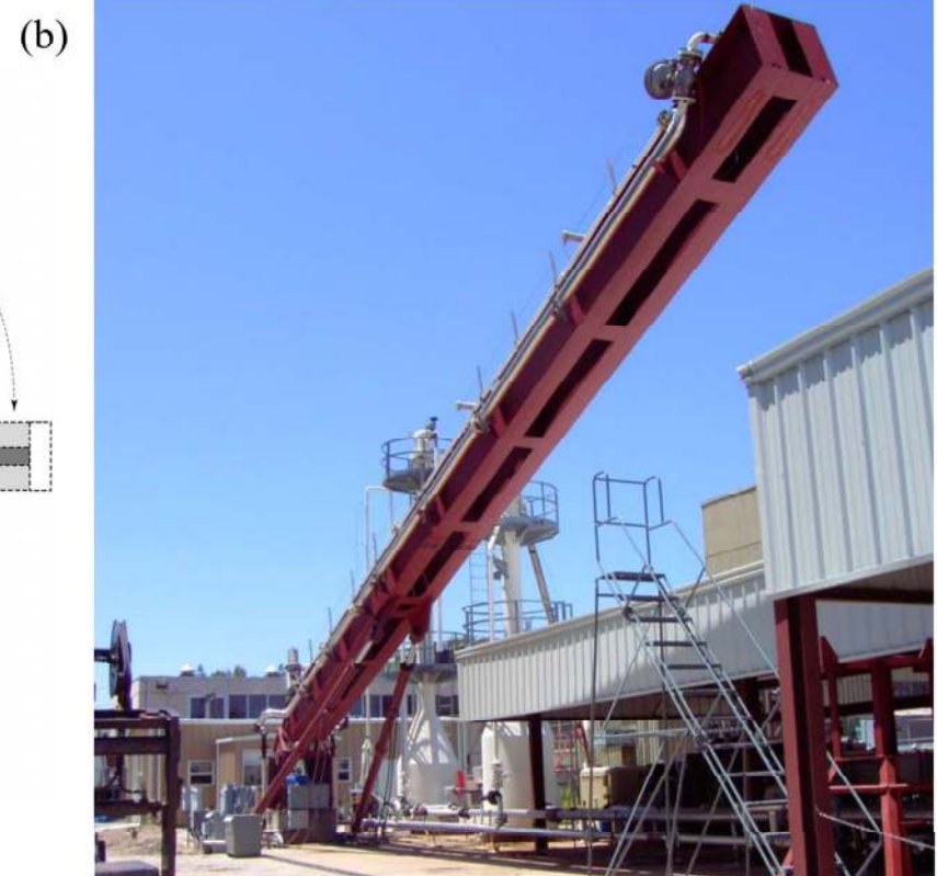
Figure 10: Typical components of an experimental set-up for cuttings transport (a); 180 Experimental testing facility at the University of Tulsa (b). 181
