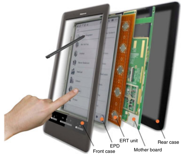
FIGURE 32 — Hanvon's dual-mode (pen and finger) digitizer combines their electromagnetic resonance digitizer with an array of pressure-sensing piezo-capacitors in the same plane as the electromagnetic resonance sensor (labeled "Electromagnetic Resonance Technology (ERT) unit"). The piezo-capacitors enable sensing finger pressure through the electronic paper display (EPD) typically used in an e-reader. Source: Hanvon.
