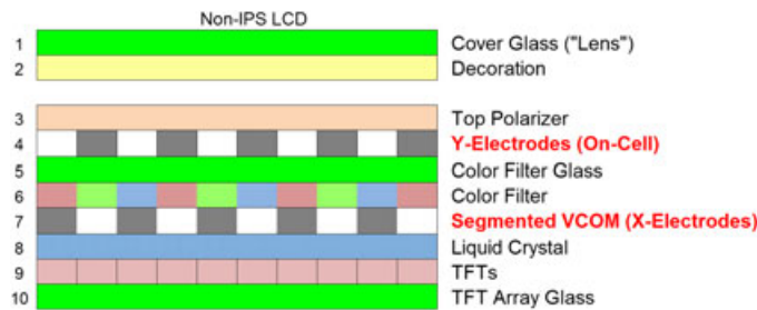
FIGURE 23 — A “true mutual-capacitance hybrid on-cell/in-cell” touch system in a Vertical Alignment Liquid Crystal Display (VA LCD) uses on-cell Y-electrodes with exactly the same function and location as standard on-cell (row 4), whereas the X-electrode is formed by segmenting the existing Voltage Common (VCOM) layer on the inside of the color filter glass (row 7). Because the VCOM layer becomes dual purpose, this architecture requires integration of the touch controller and LCD driver. TFT, thin film transistor. Source: the author.
