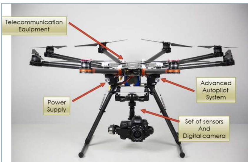
Figure 4 UAV equipped with the digital camera and set of sensors Source: Hristov, Zahariev and Beloev
