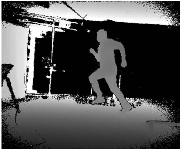
Fig. 2 Example of a depth map. Brighter pixels are further away from the camera. Black pixels are either too far away or on objects that do not reflect near infrared light
