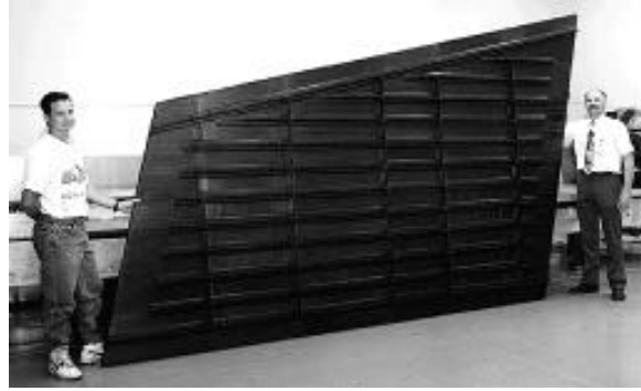
Fig. 10. Stitched/resin film infused wing stub box cover panel.
