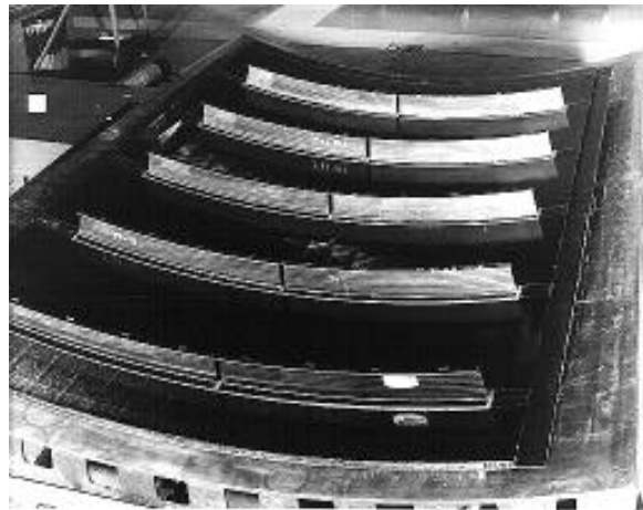
Fig. 6. Curved textile frames for fuselage keel structure.
