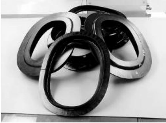
Fig. 7. Braided and woven fuselage window frames.
