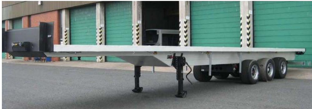
Fig. 26: World's first lightweight and aerodynamic thermoplastic composite trailer. Reproduced from ref. 219. 52x18mm (600 x 600 DPI)
