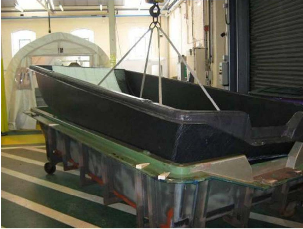
Fig. 27: Flat bottom boat case study manufactured from pCBT/GF composite and a balsa-cored sandwich panel. Reproduced from ref. 219. 112x84mm (600 x 600 DPI)
